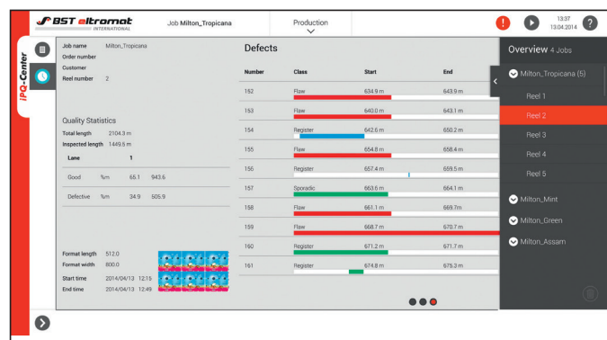
The roll logs of the Event include, amongst others, information on the error class and the running meters.
