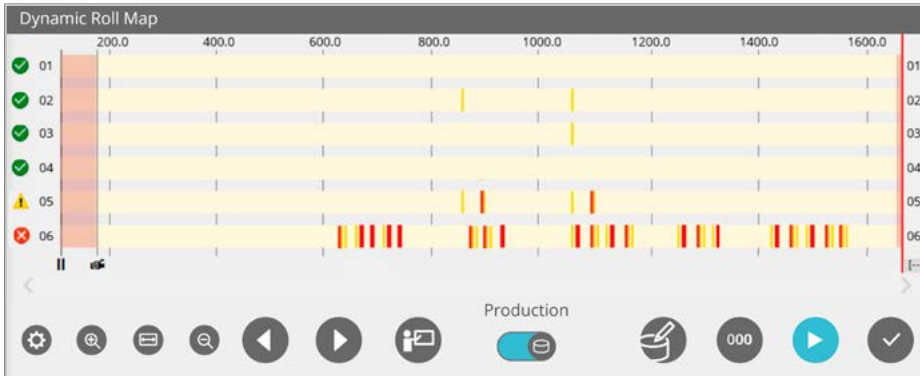
Dynamic rollmap to display the errors detected within the currently produced roll
