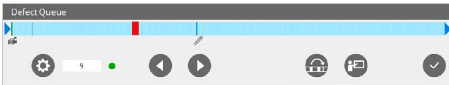
The placement control enables precise positioning of a selected defect on the rewinder or doctor machine
